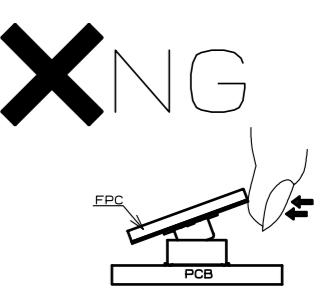
(3) If the FPC is not rigid, the connector can be broken. Please check the action of the FPC to be used repeatedly at the time of trial production. Be careful to un-mate them from the pitch direction, pulling it from the corner can also risk to putting stress on contacts.
