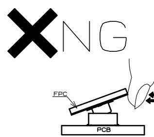
(3) IF THE FPC IS NOT RIGID, THE CONNECTOR CAN BE BROKEN. PLEASE CHECK THE ACTION OF THE FPC TO BE USED REPEATEDLY AT THE TIME OF TRIAL PRODUCTION. BE CAREFUL TO UN-MATE THEM FROM THE PITCH DIRECTION.
