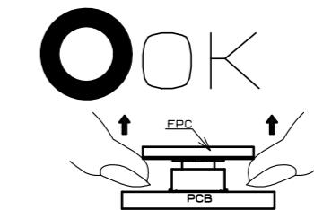
(2) IF THE CONNECTOR CANNOT BE UN-MATED PARALLEL IT CAN BE REMOVED DIAGONALLY FROM THE PITCH DIRECTION.
