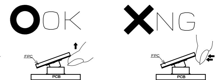
(3) IF THE FPC IS NOT RIGID, THE CONNECTOR CAN BE BROKEN. PLEASE CHECK THE ACTION OF THE FPC TO BE USED REPEATEDLY AT THE TIME OF TRIAL PRODUCTION. BE CAREFUL TO UN-MATE THEM FROM THE PITCH DIRECTION.
