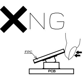
(3) If the FPC is not rigid, the connector can be broken. Please check the action of the FPC to be used repeatedly at the time of trial production. Be careful to un-mate them from the pitch direction, pulling it from the corner can also risk to putting stress on contacts.
