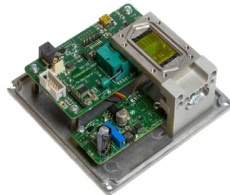
ATR spectroscopy is one method for analysing the infra-red spectrum absorbance of liquids. It provides a very simple way to sample liquids onto the sample surface of the ATR spectrometer and quickly take measurements.
