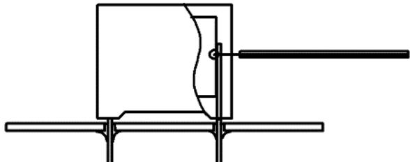
Temperature monitored inside the capacitor.
