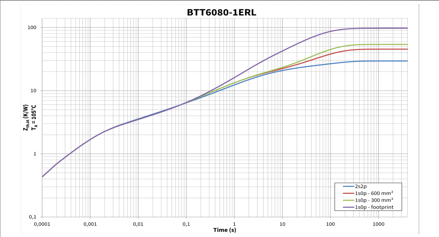
Figure 7 Typical Thermal Impedance. 2s2p set-up according Figure 5
