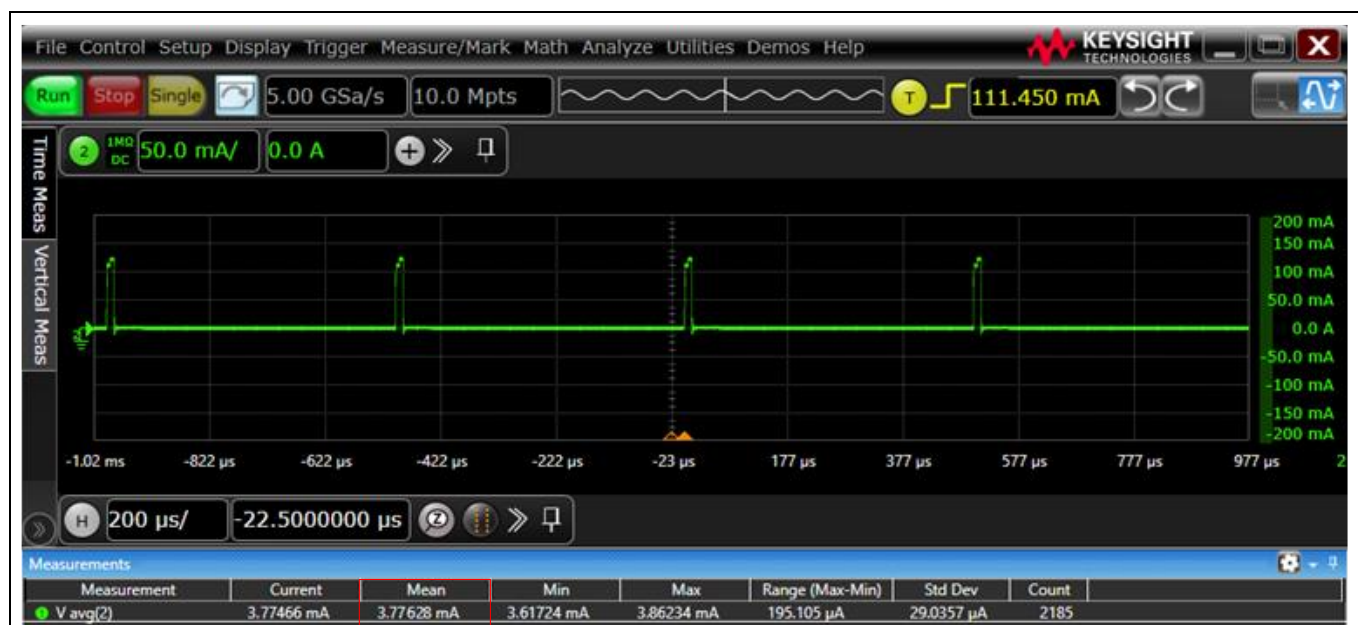
Figure 34 Current consumption of shield with PW = 5 \mu\text{s} and PRT = 500 \mu\text{s}
