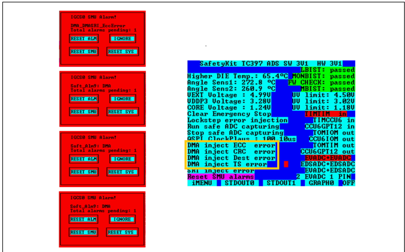
Figure 26 Application Kit Safety DMA demonstration error injection
