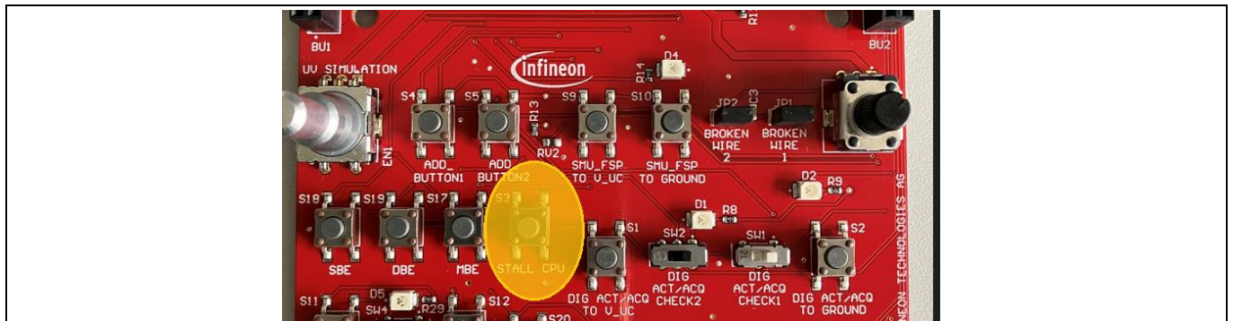
Figure 37 Stall CPU button to trigger watchdog timeout alarm
