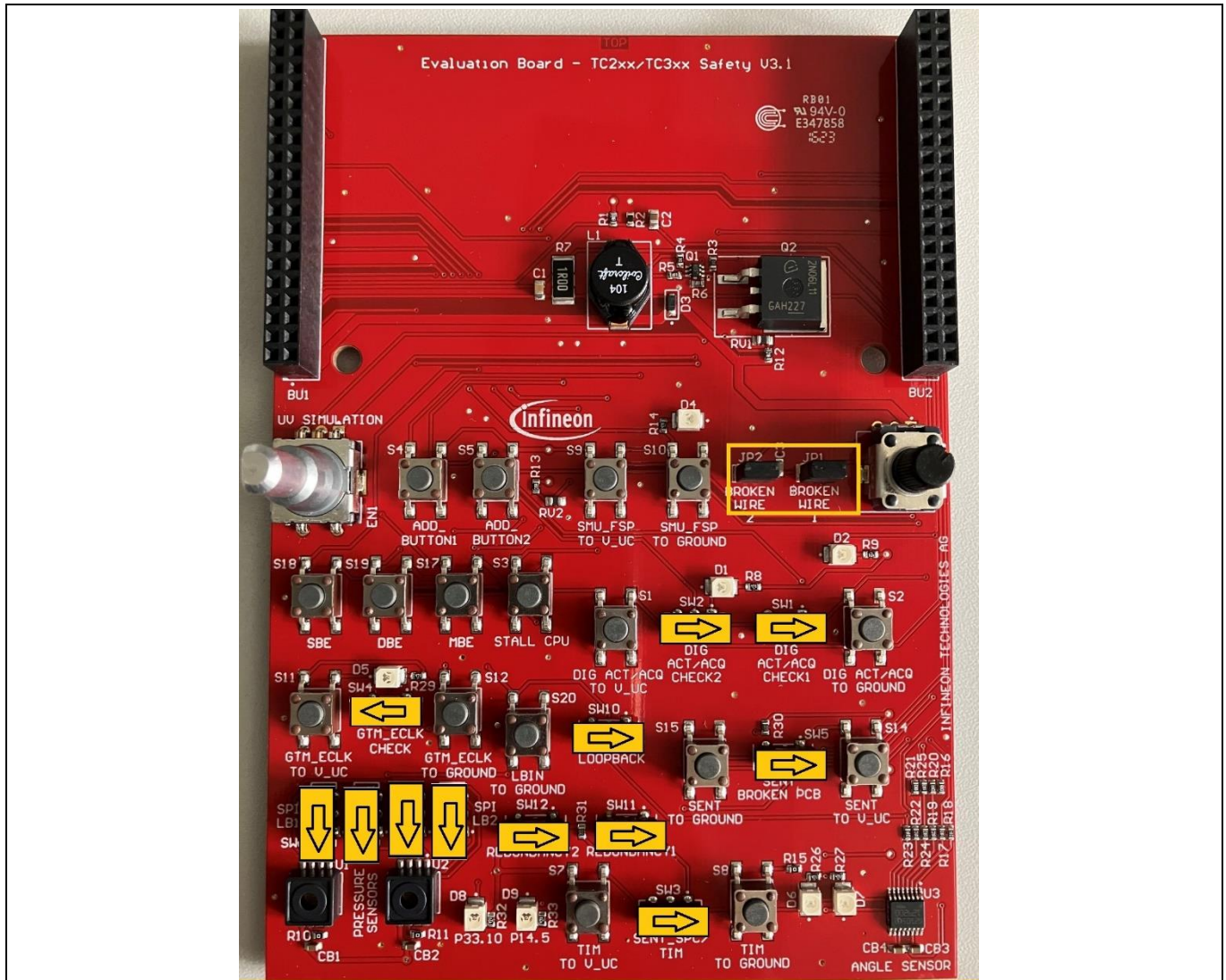
Figure 3 Default state of switches and jumper on the Evaluation Board - AURIX™ TC3xx Safety
