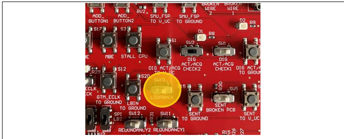
Figure 45 Port loopback switch on the Safety Evaluation Board
