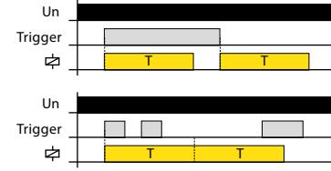
When the supply voltage is applied, the relay is open. When the control contact is closed, the relay closes and the time delay T begins. When the control contact is opened, the relay opens and the time delay T begins. If the control contact is open during timing, the relay remains closed for 2T. When the timing is complete, the relay opens. Any other change of control contact status during timing is ignored.
