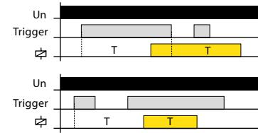
When the supply voltage is applied, the relay is open. If control contact is closed, time delay T starts. When the control contact is opened, a new time delay T begins. If the control contact is open during timing, the relay closes at the end of the timing and opens the relay after the new time delay. Any other change of control contact status during timing is ignored.
