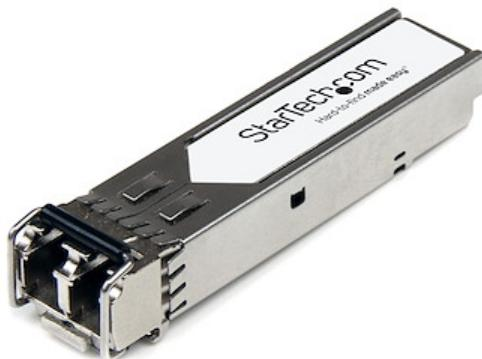
The XBR-000180-ST is a Brocade XBR-000180 compatible fiber transceiver module that has been designed, programmed and tested to work with Brocade brand switches and routers. It delivers dependable 10 GbE connectivity over fiber cable, for 10GBASE-SR compliant networks, with a maximum distance of up to 300 m (984 ft).
