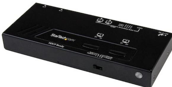
Save time and hassle by automatically switching between your HDMI audio/video sources, using the VS222HDQ 2X2 HDMI Matrix Switcher. This easy-to-use HDMI Matrix switch ensures seamless transition while switching video and display sources, with EDID copy maintaining your video resolution.
