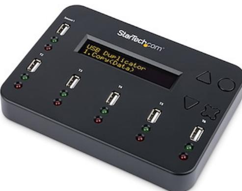
The USBDUP15 OnetoFive USB flash drive duplicator and eraser lets you quickly clone up to five backups of a single USB flash drive, or securely erase up to five flash drives, without connecting to a host computer.
