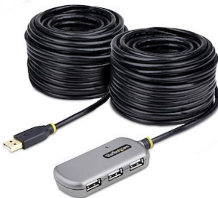
The 4-Port USB 2.0 Extension Cable (78.7ft/24m) enables multiport connectivity at distances that exceed standard USB 2.0 distance and power source limitations. Daisy chain two USB active extension cables for a maximum range of 157.4ft (48m).
