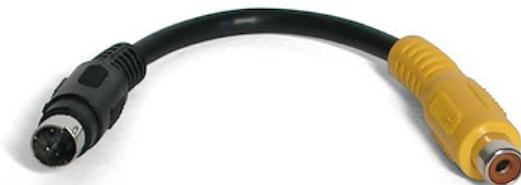
This S-Video to Composite Video Adapter features a 4-pin mini-DIN S-Video Male connector and an RCA female connector, allowing you to connect a device with S-Video output to a device with RCA Composite Video input.
