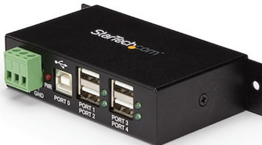
This TAA compliant 4-port industrial USB 2.0 hub gives you the scalability you need in harsh industrial environments, product and repair labs, conference rooms or office workstations. With its rugged industrial grade metal housing, it is designed to meet the advanced requirements of connecting a high number of devices in factories and office environments.
