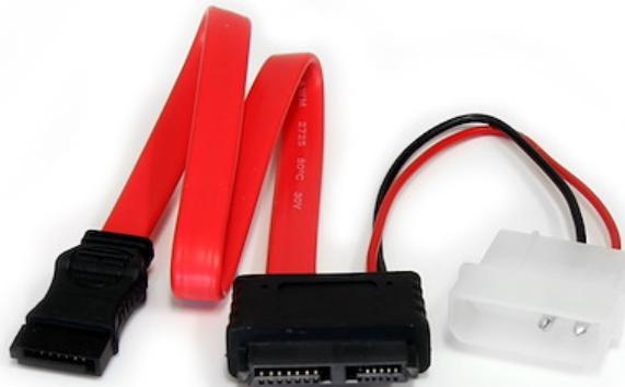
The SLSATAF12 Slimline SATA to SATA with LP4 Power Cable (12-inch) features a SATA data receptacle and a LP4 power connection on one end, and a Slimline Serial ATA receptacle on the other - allowing you to connect a slim SATA drive to a computer motherboard that does not have a Slimline connection available.
