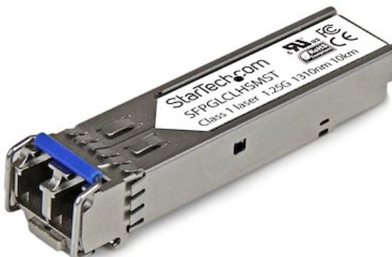
The SFPGLCLHSMST is a Cisco GLC-LH-SM compatible fiber transceiver module that has been designed, programmed and tested to work with Cisco brand switches and routers. It delivers dependable 1GbE (1000 Mbps) connectivity over fiber cable, for 1000BASE-LX/LH compliant networks, with a maximum distance of up to 10 km (6.2 mi).
