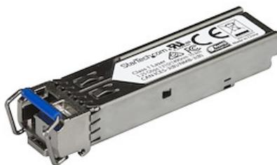
The SFPGE10KT3R4 is a Juniper SFP-GE10KT13R14 compatible fiber transceiver module that has been designed, programmed, and tested to work with Juniper brand switches and routers. It delivers dependable 1 GbE connectivity over fiber cable, for 1000BASE-BX10-U compliant networks, with a maximum distance of up to 10 km (6.2 mi).
