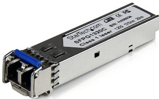
The SFPG1320C is a Cisco GLC-LH-SMD compatible fiber transceiver module that has been designed, programmed and tested to work with Cisco brand switches and routers. It delivers dependable 1 GbE connectivity over fiber cable, for 1000BASE-LH compliant networks, with a maximum distance of up to 20 km (12.4 mi).
