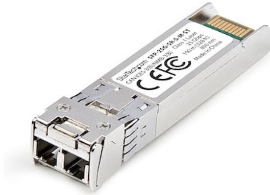
MSA-compliant fiber optic transceiver with 25Gbps connectivity and up to 100m (328ft) over LC-terminated Multimode Fiber (MMF) cable. The optical module has been programmed and tested for seamless integration with MSA-compatible switches and routers to ensure compatibility and reliability.
