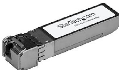
The SFP-10GB-BX-D-20-ST is a MSA Compliant downstream fiber SFP+ transceiver which pairs with StarTech.com's SFP-10GB-BX-U-20-ST. They are designed, programmed and tested to work with 10GBASE-BX compatible MSA Compliant switches and routers. The SFP+ transceiver module supports a maximum distance of up to 20 km (12.4 mi) and delivers dependable 10 GbE connectivity over fiber cabling.
