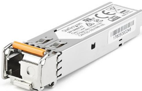
The SFP1GBX10DES is a Dell EMC SFP-1G-BX10-D compatible downstream fiber SFP transceiver which pairs with StarTech.com's SFP1GBX10UES. They are designed, programmed and tested to work with 1000BASE-BX10 compatible Dell EMC switches and routers. The SFP transceiver module supports a maximum distance of up to 10 km (6.2 mi) and delivers dependable 1 GbE connectivity over fiber cabling.
