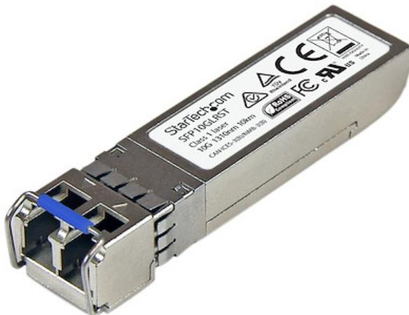
The SFP10GLRST is a Cisco SFP-10G-LR compatible fiber transceiver module that has been designed, programmed and tested to work with Cisco brand switches and routers. It delivers dependable 10 GbE connectivity over fiber cable, for 10GBASE-LR compliant networks, with a maximum distance of up to 10 km (6.2 mi).
