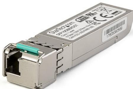
The SFP10GBX10US is a Dell EMC SFP-10G-BX10-U compatible upstream fiber SFP transceiver which pairs with StarTech.com's SFP10GBX10DS. They are designed, programmed and tested to work with 10GBASE-BX10 compatible MSA switches and routers. The SFP+ transceiver module supports a maximum distance of up to 10 km (6.2 mi) and delivers dependable 10 GbE connectivity over fiber cabling.
