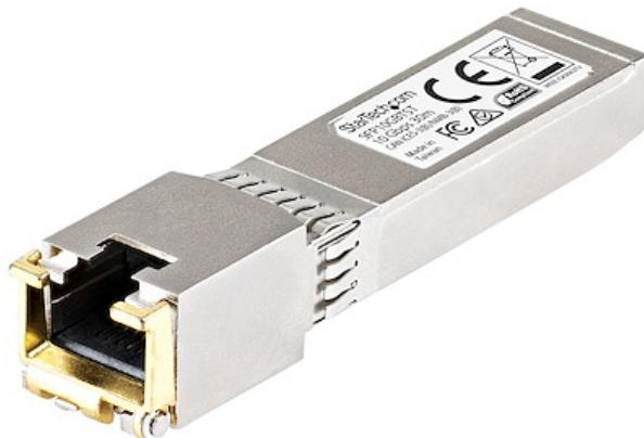
The SFP10GBTCST is a Cisco compatible copper transceiver module that has been designed, programmed and tested to work with Cisco brand switches and routers. It delivers dependable 10 GbE connectivity over copper cable, for 10GBASE-T compliant networks, with a maximum distance of up to 30 m (98.4 ft).
