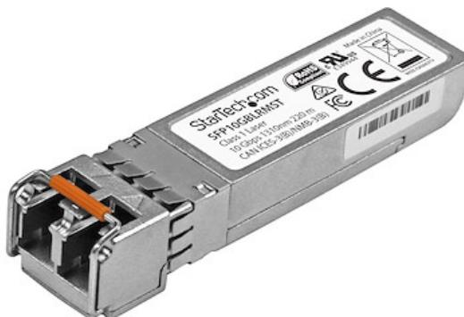
The SFP10GBLRMST is an MSA compliant fiber SFP transceiver that's designed, programmed and tested to work with 10GBASE-LRM compatible MSA switches and routers. The SFP+ transceiver module supports a maximum distance of up to 220 m (721 ft.) and delivers dependable 10 GbE connectivity over fiber cabling. **Technical Specifications:**
