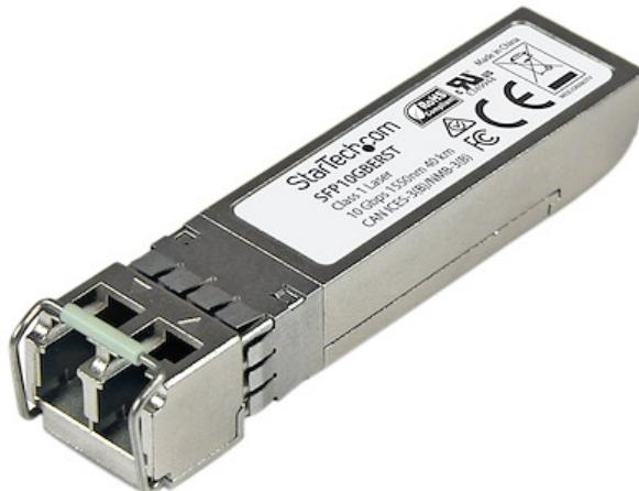
The SFP10GBERST is an MSA compliant fiber SFP transceiver that's designed, programmed and tested to work with 10GBASE-ER compatible MSA switches and routers. The SFP+ transceiver module supports a maximum distance of up to 40 km (24.8 mi) and delivers dependable 10 GbE connectivity over fiber cabling. **Technical Specifications:**
