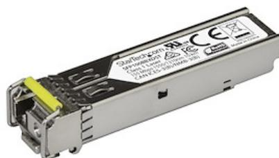
The SFP100BBXDST is an MSA compliant downstream fiber SFP transceiver which pairs with StarTech.com's SFP100BBXUST. They are designed, programmed and tested to work with 100BASE-BX compatible MSA switches and routers. The SFP transceiver module supports a maximum distance of up to 10 km (6.2 mi) and delivers dependable 1 GbE connectivity over fiber cabling. <b>Technical Specifications: </b>
