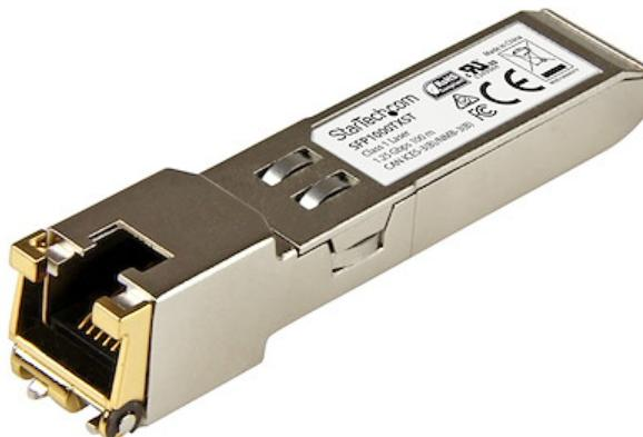
The SFP1000TXST is an MSA compliant copper SFP transceiver that's designed, programmed and tested to work with 1000BASE-TX compatible MSA switches and routers. The SFP transceiver module supports a maximum distance of up to 100 m (328 ft) and delivers dependable 1 GbE connectivity over copper cabling. **Technical Specifications:**
