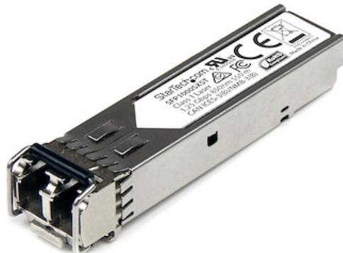
The SFP1000SXST is an MSA compliant fiber SFP transceiver that's designed, programmed and tested to work with 1000BASE-SX compatible MSA switches and routers. The SFP transceiver module supports a maximum distance of up to 550 m (1804 ft) and delivers dependable 1 GbE connectivity over fiber cabling. **Technical Specifications:**
