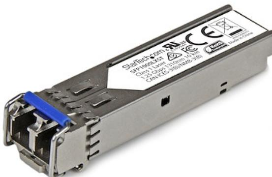
The SFP1000LXST is an MSA compliant fiber SFP transceiver that's designed, programmed and tested to work with 1000BASE-LX compatible MSA switches and routers. The SFP transceiver module supports a maximum distance of up to 10 km (6.2 mi) and delivers dependable 1 GbE connectivity over fiber cabling. **Technical Specifications:**
