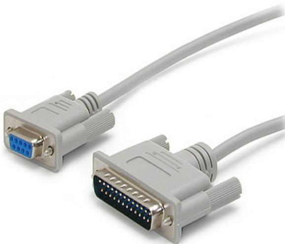
The SCNM925FM 10ft Cross Wired Serial/Null Modem Cable features one DB9 female and one DB25 male connector, allowing you to connect a 9-pin serial device to a 25-pin serial port, or transfer files from PC-to-PC via a serial connection.
