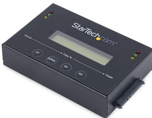
The SATDUP11 standalone hard drive duplicator eraser enables you to copy 1-to-1, or erase up to 2 SATA hard drives simultaneously without a host computer.
