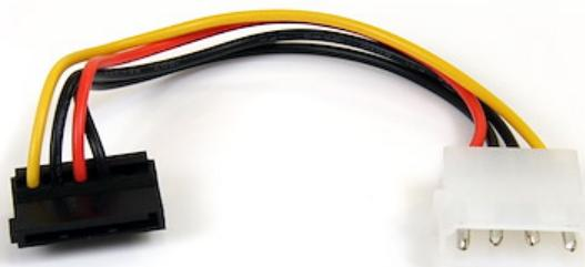
This 6-inch 4-Pin LP4 to Right Angle SATA power adapter features one 4-Pin LP4 male connector and one (female) right angle SATA power connector, allowing you to power a Serial ATA hard drive from a conventional LP4 connection, eliminating the need to upgrade the computer power supply for compatibility with the SATA hard drive.
