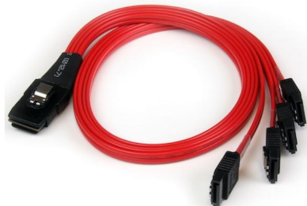
The SAS8087S4R50 SFF-8087 to 4x SATA Reverse cable features one 36-pin plug (SFF-8087), which fans out to four SATA 7-pin receptacles, providing a reliable solution for connecting a Mini SAS backplane to a SAS / SATA RAID controller or motherboard.
