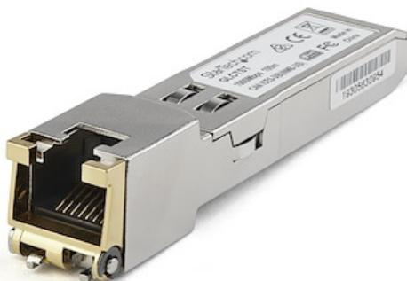
The RXGETSFPST is a Juniper RX-GET-SFP compatible copper transceiver module that has been designed, programmed and tested to work with Juniper brand switches and routers. It delivers dependable 1 GbE connectivity over copper cable, for 1000BASE-T compliant networks, with a maximum distance of up to 100 m (328 ft).
