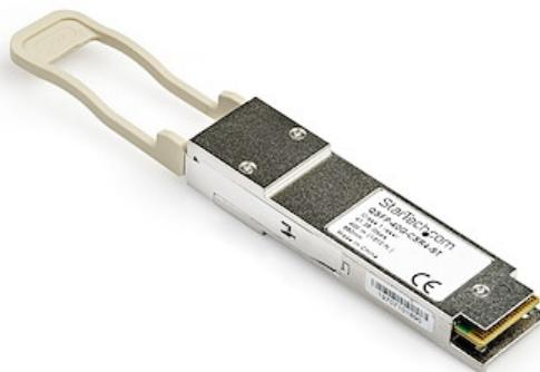
The QSFP-40G-CSR4-ST is a Cisco QSFP-40G-CSR4 compatible fiber transceiver module that has been designed, programmed and tested to work with Arista Networks brand switches and routers. It delivers dependable 40 GbE connectivity over fiber cable, for 40GBASE-SR4 compliant networks, with a maximum distance of up to 400 m (1312 ft.).
