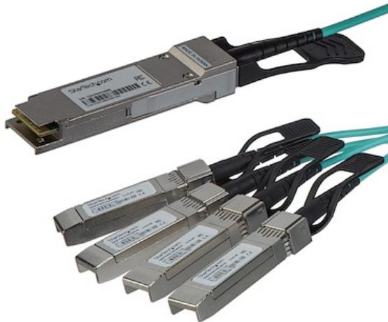
The QSFP4X10GAO3 is a Cisco QSFP-4X10G-AOC3M compatible optical quad small form-factor pluggable (QSFP+) breakout cable that is designed, programmed and tested to work with Cisco brand compatible servers or routers and complies with MSA industry standards. Connecting a single QSFP+ port (40 GbE) to four 10G SFP+ ports, this active optical breakout cable is fully hot-pluggable which makes upgrades and replacements seamless by minimizing network disruptions.
