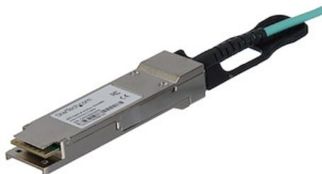
The QSFP40GAO30M is an MSA compliant optical quad small form-factor pluggable (QSFP+) cable that is designed, programmed and tested to work with 40 GbE compatible switches and routers. This AOC QSFP+ cable supports 40 Gigabit Ethernet applications (4 x 10GbE) connected through QSFP+ ports. It is a low-power, low-latency cable that is hot-swappable, making upgrades and replacements seamless by minimizing network disruptions.
