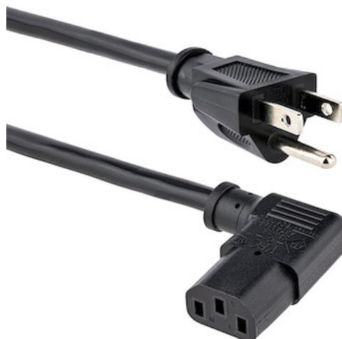
This 6ft Right Angle Power Cord features a standard NEMA 5-15P connector as well as a right-angled C13 connector allowing you to plug a monitor, PC, or laser printer into a grounded power outlet.
