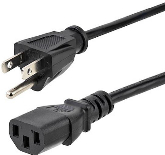
The PXT101143 NEMA 5-15P to C13 Computer Power Cord (3ft) features 14 AWG wire suitable for high power connections, making it a reliable solution for large server applications that require a higher rated, heavier gauge cable, and connecting to Power Distribution Units (PDU).
