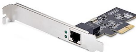
This 2.5 GbE network interface card (NIC) features an Intel I225-V chipset with Intel vPro technology, to enhance performance and data integrity. Variable multispeed options (2.5/1Gbps and 100/10Mbps) enable support for both new and legacy network hardware. Leverage existing Cat5e or CAT6 cabling infrastructure while adding NBASE-T (802.3bz) compatibility for seamless integration.
