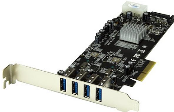
The PEXUSB3S42V 4-Port PCI Express PCIe SuperSpeed (5Gbps) USB 3.0 Card Adapter lets you add four USB 3.2 Gen 1 ports with two dedicated 5 Gbps channels to your PCIe x4-enabled PC. This independent port architecture improves USB 3.2 Gen 1 performance by transferring data on two individual channels to your computer, giving you faster file transfers.
