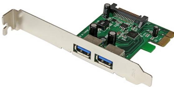
The PEXUSB3S24 2-Port PCI Express USB 3.2 Gen 1 Card lets you add two USB 3.2 Gen 1 ports to your PCI Express-enabled computer system, with an optional SATA power connector to connect to your system power supply and deliver up to 900mA of power per port to USB 3.2 Gen 1 bus-powered devices (500mA for USB 2.0).
