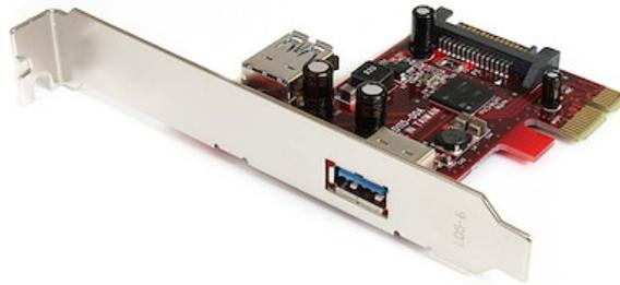
The PEXUSB3S11 PCI Express USB 3.2 Gen 1 Card lets you add one internal, and one external USB 3.2 Gen 1 port to your PC through a PCI Express slot.
