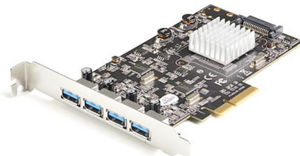
This PCIe USB 3.2 Gen 2 controller card installs into an available PCI-Express x4 slot in your computer and enables you to upgrade your current system by adding four SuperSpeed USB-A (10Gbps) ports. The card features dual ASM3142 controllers with up to 20 Gbps of total bandwidth shared across all 4 ports.
