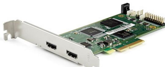
You can install the HDMI capture card into any low-profile or full-profile PCIe slot, including fixed workstations such as 2U or 4U rack-mounted servers or media centers.
