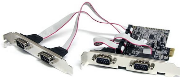
The PEX4S553 4-Port Native PCI Express RS232 Serial Adapter Card with 16550 UART lets you add 4 RS232 (DB9) serial ports, using a single PCI Express expansion slot.
