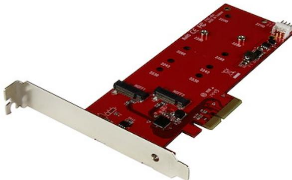
This M.2 SSD controller card lets you install two M.2 SATA solid-state drives (SSD) into your PC through PCI Express. You can mount virtually any M.2 drive directly to the card, giving you a convenient and discreet way to improve your computer system performance. Plus, the card is a vital computer add-on if you need to recover data from an existing M.2 drive, or for expanding your overall internal storage.
